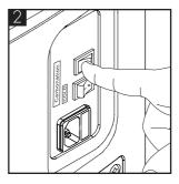
After completing the water installation, turn on the soda power switch and the pump will run. Do not open the regulator valve until the carbonated switch has been turned on.
