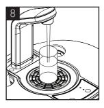
Preflush the new filter to waste using the ambient button until the water appears clear and is free of air. Flush through a small amount of water to check all functions.
