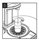
When the external cleaning (minimum 5 minutes) is completed, flush the machine using the cold button with clean water until the dispense water runs clear. Repeat briefly with the ambient button (and sparkling button if present).
