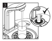
The tank is empty of sparking water when only CO2 is being released.
