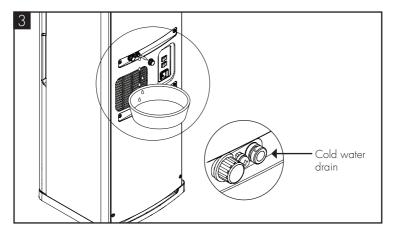
To drain the Direct Chill tank, remove the cap on the back of the machine. We recommend it is refitted immediately upon draining being completed.
