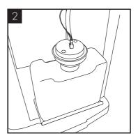
Locate and connect the drainage tubing into the top of the level sensor connector.
