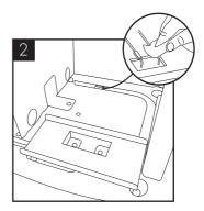
Locate the leak and rectify. Locate the detection probe which can be found in the bottom at the rear of the machine. Dry the probes and internal area with a dry cloth.
