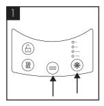
Briefly press cold/ambient dispense button to release internal water pressure from the machine. Remove the existing filter.
