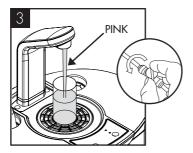
Turn on incoming water, allow service cartridge to fill. Dispense water using the cold button until the water appears pink. Briefly press the ambient button too. Repeat with sparkling button if present.
