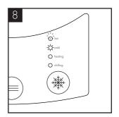
When the heating LED is off the pre-set temperature has been reached. This can take up to 30 minutes.
