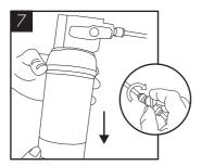
Turn off water and remove the service filter. Retain service filter for reuse. Fit new filter. Turn on incoming water supply.
