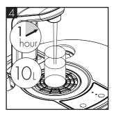
Flush through approximately 10 litres of water. Check and adjust the CO2 pressure accordingly. The machine needs leaving for 1 hour for sparkling water to develop.
