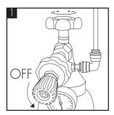
Attach the regulator to the disposable CO2 bottle, ensuring the regulator is closed. Connect the CO2 bottle and regulator to the machine using 1/4 inch pipe.
