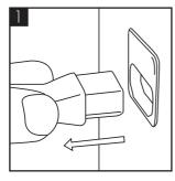
Please make sure the machine is completely disconnected from electricity before carrying out any maintenance work.
