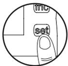
1. Press and hold the 'Set' button until CP shows on the display – Release the button.
