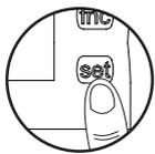
1. Switch on Mains power – the display will flash several times, then the fridge system will switch on and the display will give a steady reading, this is the temperature of the water bath sensor.
