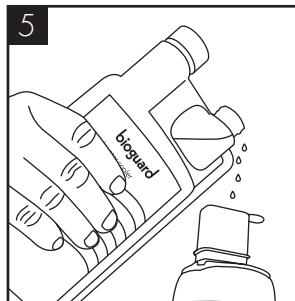
5 Add 25 ml of Bioguard Internal Sanitisation fluid to a clean and empty service filter cartridge.
