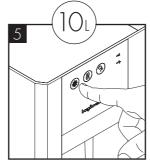
Flush through approximately 10 litres of water. Check and adjust the CO2 pressure accordingly.
