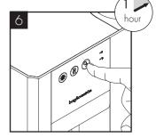
It will be necessary to leave the machine for up to 1 hour for sparkling water to develop, by absorbing the CO2.
