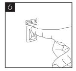
To avoid damage do not turn on the cold power switch until water flows out of the machine.
