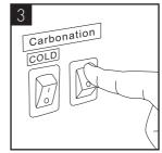
On sparkling models turn on the carbonation switch on the back of the unit.
