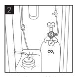
Connect the assembled CO2 bottle and regulator to the machine using 1/4 inch pipe.
