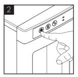
All hot & non sparkling cold tanks must be purged of air by holding the corresponding button.
