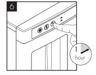
It will be necessary to leave the machine for up to 1 hour for sparkling water to develop, by absorbing the CO2.
