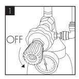
Attach the regulator to the disposable CO2 bottle, ensuring the regulator is closed.
