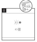
When the cold water switch is turned on, the cold water indicator will be lit.
