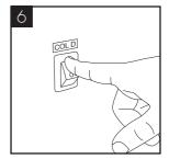
To avoid damage do not turn on the cold power switch until water flows out of the machine. (If applicable)
