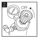
Attach the regulator to the CO2 bottle, ensuring the small pressure relief vent in the stem is facing away from you or anyone else. Ensure the regulator is closed. Hand tighten securely.
