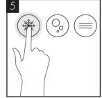
For any units you wish to not be triggered by the waste kit turn off the bluetooth on the unit by pressing the chilled icon 4 times and hold on the 5th press.
