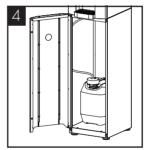
Ensure the drip tray is securely fitted. For base cabinets feed drain pipe down the side. Fit pipe to level sensor and waste container.
