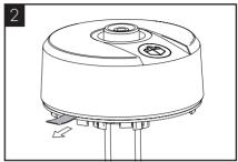
Remove the pull tabs under the batteries on the level sensor module. Once removed the level sensor will connect to all bluetooth units within a small area. If multiple level sensors are used only the closest unit to the level sensor will be triggered.
