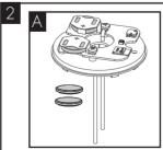
2A - Replace both batteries with correct orientation. Replace cover when complete.
