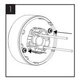
For battery removal and buzzer control, unscrew the two screws on the under side and remove the top cover.
