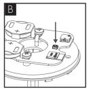
2B - Turn buzzer off or on by pressing button on the board. Replace cover when complete.
