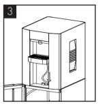
Remove the standard drip tray or drip tray plug from the unit. Replace with the new tray and feed the pipe through the unit and base cabinet or counter top.
