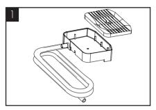
Select the correct drain kit for the unit you want to connect the waste kit to. Connect the new or existing drip dray to the waste pipe both provided in the kit and replace any fonts if required.
