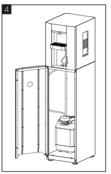
To fit the optional drain kits remove the original drip tray and feed the pipe, fitted on the new drip tray, through the hole in the e4/e6 unit and base cabinet. Feed the pipe down the left hand side of the cabinet and fit to optional Bluetooth Alarmed Waste Kit (720400) or to an external drain.
