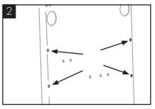
If it is more practical to mount the unit to a wall use the optional wall bracket set (194107) with the holes on the back of the cabinet.
