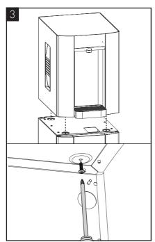
Place the unit on the base cabinet in the feet indents on the top of the cabinet. To secure the unit to the base cabinet use the four screws provided. Fix through from the inside of the base cabinet up in to the feet of the unit.
