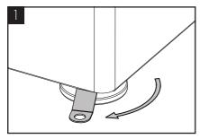
Remove the rear feet and fit the brackets as provided onto them and refit. Adjust the level of the unit by winding or unwinding the feet. Once the base cabinet is in the suitable position fix the brackets into place through the floor.
