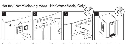
Connect the unit to the electricity supply and ensure unit is switched on.
