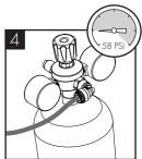
Stand the cylinder in a suitable place. We recommend between 3.5 - 4 bar (58 PSI) (max). Do not exceed 4 bar pressure.
