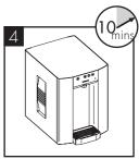
Allow the machine to stand for 10 minutes for the initial chilling and heating process to complete.
