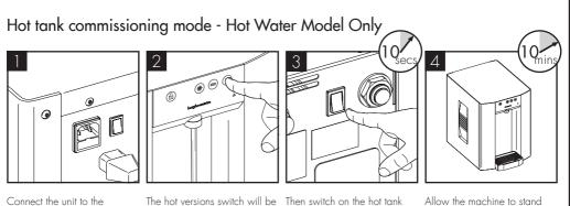
Connect the unit to the electricity supply and ensure unit is switched on.
