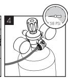
Stand the cylinder in a suitable place. We recommend between 3.5 - 4 bar (58 PSI) (max). Do not exceed 4 bar pressure.
