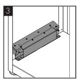
Take the sensorbeam and fix to the cabinet base using the m4 fixing screws provided and pass the wiring harness through the back of the cabinet.
