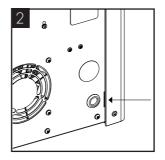
Remove the existing closed grommet located on the bottom right of the backplate.
