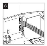
For E4 connect the harness to the back of the HMI as shown.
