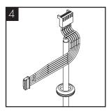
Push the supplied open grommet over the wiring harness connections and fit into the backplate hole as previous.
