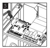
For E6 plug into the board labelled 'Foot Switch' as shown.
