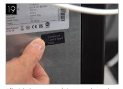
Affix label to reverse of dispenser, located below the rating plate as shown, to indicate that the compressor control board is fitted.
