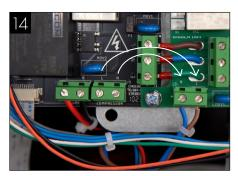
Place the now released, Live and Neutral compressor power wires into the terminal on the compressor control board, ensuring correct placement of Neutral and Live wires as indicated on the board.
