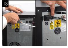
Re-install the top panel. Reconnect and power on the unit. You should be able to hear the compressor and fan running.
